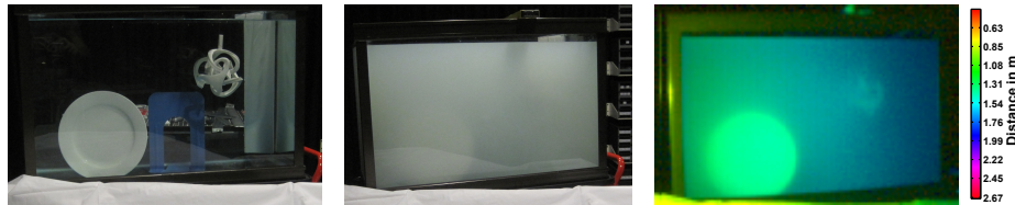
Fig. 1. Example of imaging in scattering media using our approach. Left: Original scene with objects submerged in water-filled glass tank. Center: 160 ml milk added. Right: Objects that are “invisible” due to strong scattering, like the structured object on the top right or parts of the circular object become detectable using our approach.
