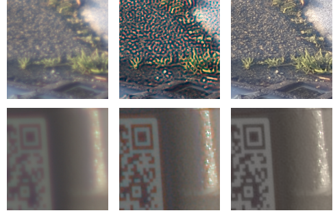
Fig. 5. Effect of using the cross-channel priors (with the addition from Sec. 5.5) for two image patches (full images in results section). Left: Original blurred capture. Middle: Independently deconvolved results for each channel using the method of Levin et al. [2007]. Right: Deconvolution result with our cross channel prior.
