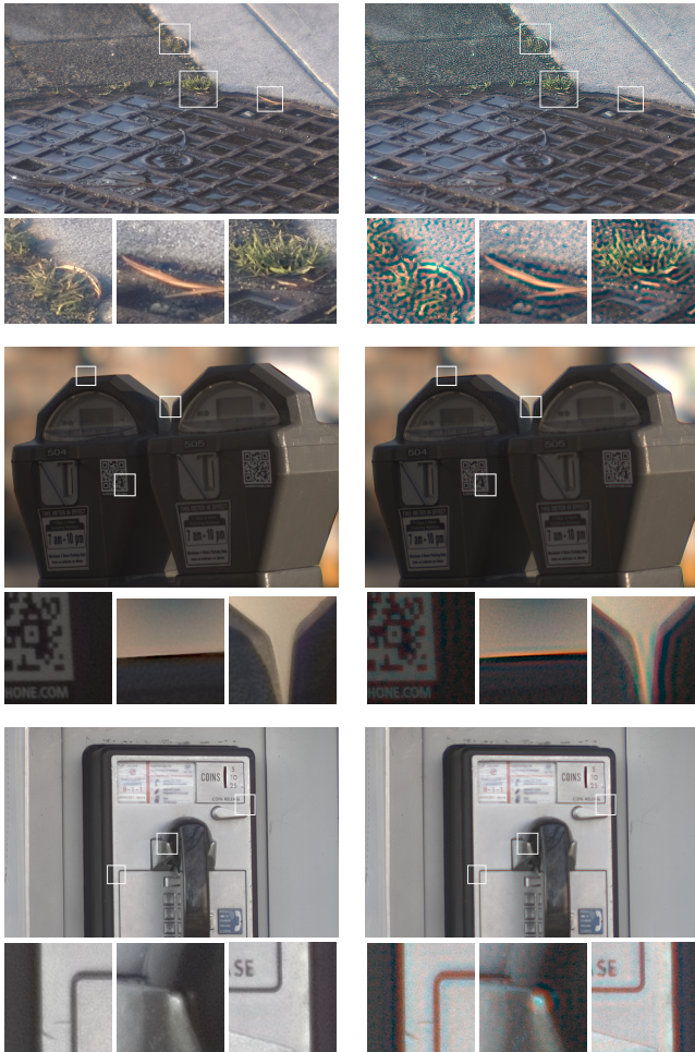
Fig. 20. Images from Fig. 11, 1 reconstructed using our cross-channel prior (left) and restored with the Yuv-regularization from [Schuler et al. 2011] (right).
