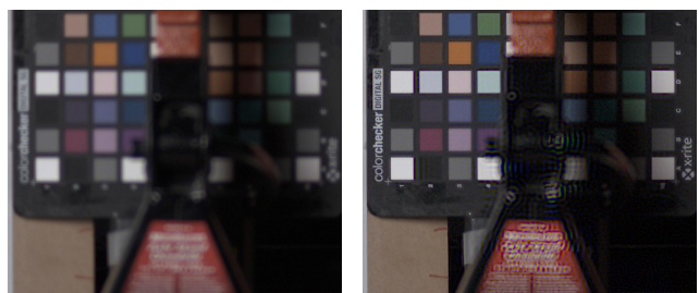
Fig. 14. Left: Captured input image from biconvex lens at f/2 . Right: Deblurred version. A very low cross-prior weight has been used here to illustrate the depth-dependency of the PSF.
