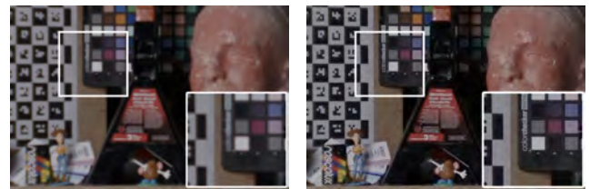
Fig. 12. Left: Cropped central region of the image from achromatic lens with f/2.0 . Right: Deblurred version.
