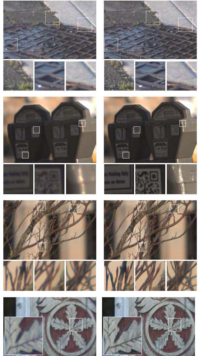
Fig. 11. Images captured with a simple plano-convex lens (left) and restored with our method (right). Note recovered spatial detail and the absence of color fringing. Also note the bokeh and graceful handling of out-of-focus blur in the top three images.
