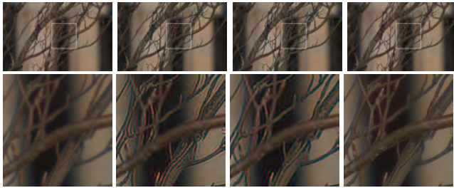
Fig. 18. Top row from left to right: Captured image, deconvolved result from [Levin et al. 2007] independently on each channel, IRLS method from [Levin et al. 2007] extended with our prior, our result. Bottom row: Patches in same order of the methods.
