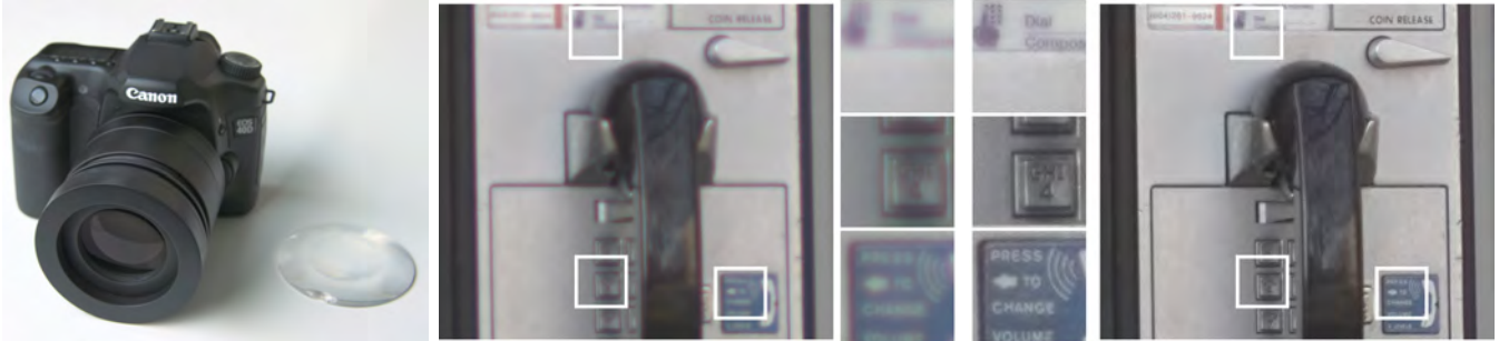
Fig. 1. Our system reliably estimates point spread functions of a given optical system, enabling the capture of high-quality imagery through poorly performing lenses. From left to right: Camera with our lens system containing only a single glass element (the plano-convex lens lying next to the camera in the left image), unprocessed input image, deblurred result.
