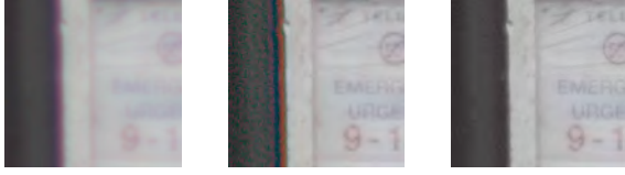
Fig. 7. Chromatic artifacts in low-intensity areas. Left: Original blurred patch. Center: Reconstruction using Eq. (9). Notice the chromatic artifacts in all low-intensity areas and the correct reconstruction in the other areas. Right: Regularization for low-intensity areas added as discussed below.
