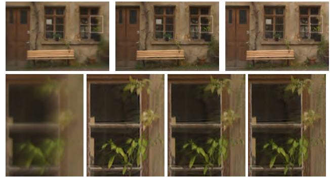
Fig. 19. Top row from left to right: Captured image, our deconvolved result, result from [Schuler et al. 2011]. Patch matrix below from top left to bottom right: Captured image, result from [Schuler et al. 2011], our result with strong regularization (smoother reconstruction), our result with low regularization (more detailed reconstruction) .
