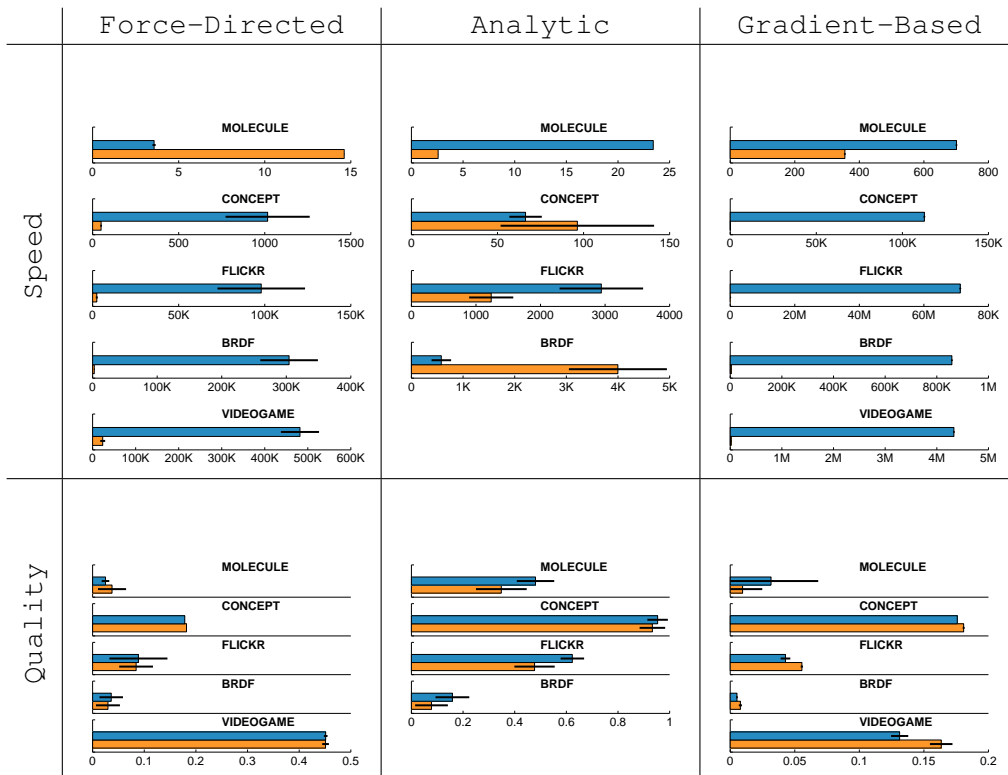
Figure 6.2: Comparison of speed (top) and quality (bottom). In each pair, the top blue bar is the original MDS algorithm, and the bottom orange bar is the Glint instantiations. The black lines indicate 95% standard error bars.
