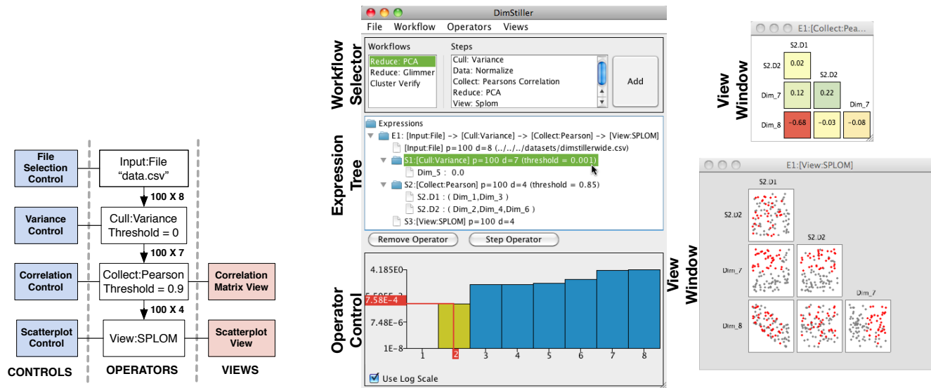
Figure 3.1: Left: The anatomy of a simple DimStiller expression. Input data is fed into a pipeline of operators that alter the dimensionality of the data. Each operator may or may not have controls or views. An Operator's control is displayed when it is selected in the Expression Tree. An operator's view is shown in a separate window, allowing side by side comparison between multiple views. Changing an operator's parameter in the control may produce a change to its output that is propagated across the expression using events that may travel both upstream and downstream from the operator. Right: The DimStiller interface for this expression, showing the Collect:Pearson and View:SPLOM views. The Cull:Variance expression is selected in the Expression Tree, so its control is visible.
