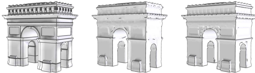
Figure 4.18: Arc de Triomphe (left). Low resolution envelope (middle) is initialized with grid size 21 \times 35 \times 33 . The construction converged in 12 iterations. High resolution envelope (right) is initialized with grid size 35 \times 61 \times 57 . The construction converged in 8 iterations.
