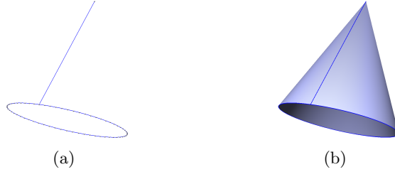
Figure 4.7: Modeling a cone by a boundary with a single dart.
