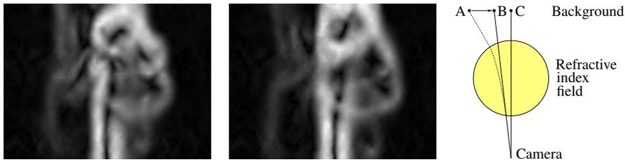
**Figure 5.3:** Candle plume results. Left and middle: magnitude plots of optical flow vectors from two consecutive images in the sequence. Right: refraction in a cylindrical lens makes the object at *A* appear where *B* did previously.
