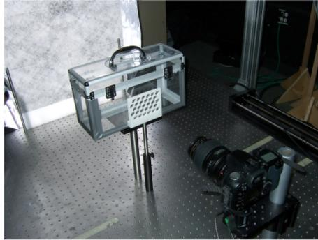
**Figure 4.3:** Lens array setup and water tank.
