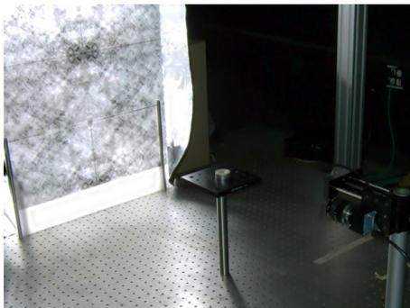
**Figure 4.1:** Standard single camera setup and small candle.
