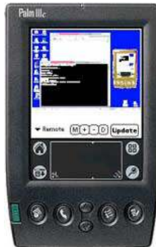
Figure 2.7. The Remote Commander full-screen view on PDA showing a screen shot of the personal computer on the display of the PDA
