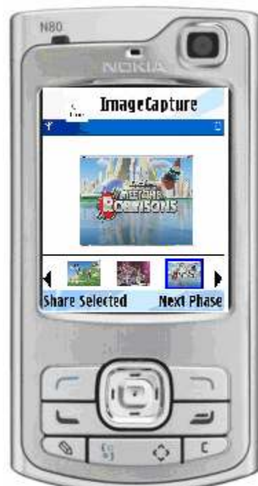
Figure 4.4. Nokia N80 mobile phone display showing interface for selecting screen shots. There are three thumbnails of the screen shots displayed underneath the currently viewed screen shot which is displayed in the center of the screen. Arrows on the bottom left and bottom right of the display indicates that there are more screen shots to view.
