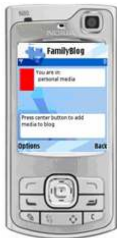
Figure 6.8. Nokia N80 mobile phone showing the screen on the phone when controlling large display. The color of the user's cursor (red) is displayed on the top left. The area which the user is controlling (personal media) is stated at the top of the display. Additional instructions are display on the bottom of the display.
