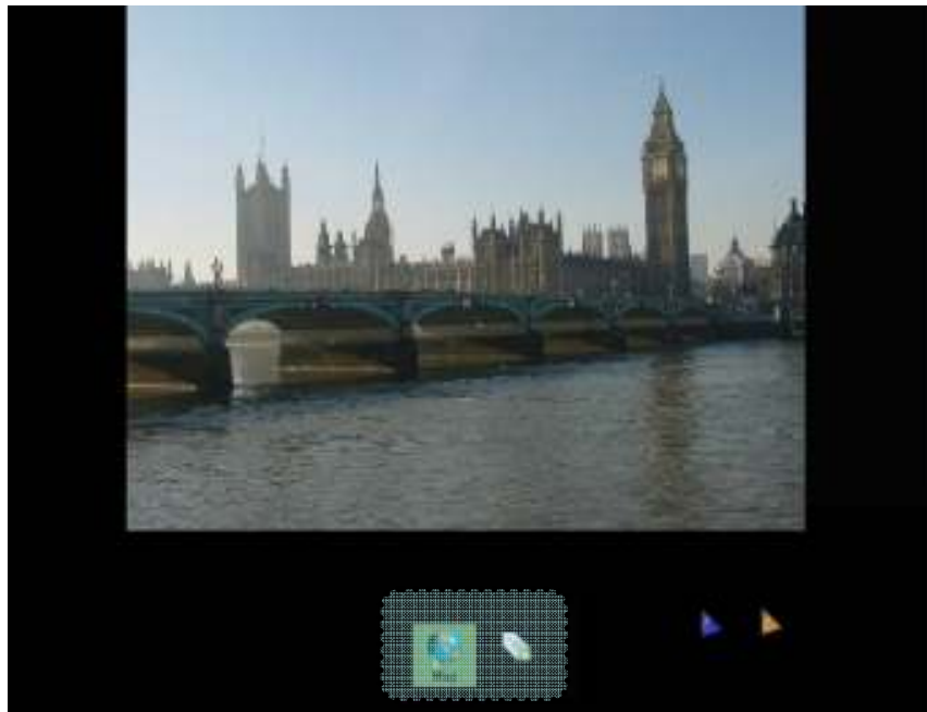
Figure 3.2. The trip planning prototype in three-quarter screen mode showing that once the Map Icon is clicked by a user the background of the Map Icon turns the same color (green) as the user's cursor (green).
