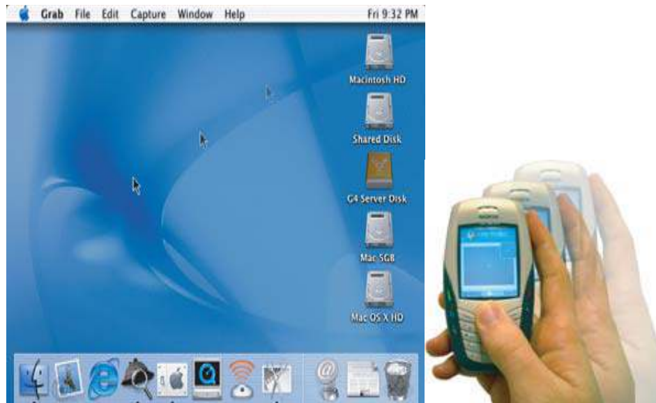
Figure 2.5. The Sweep technique can be used to control a cursor on a large display much like with an optical mouse. A user is moving the cell phone to move the cursor on the large display.
