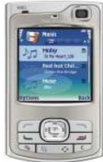
Figure 4.1. Nokia N80 mobile phone used for prototype in our study. The personal display on this phone has 352 x 416 pixels and can display up to 262,144 colors
