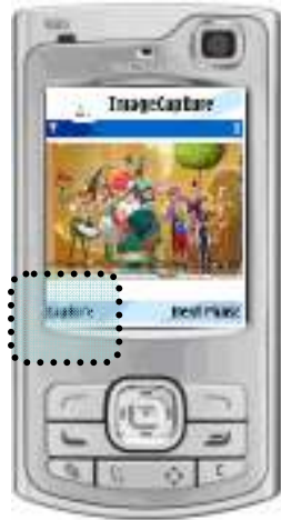
Figure D.1.1. Nokia N80 mobile phone display showing a screen shot created from the video playing on the large display. The 'Capture' button is on the bottom left of the display.
