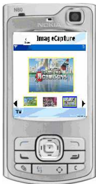
Figure D.1.15. Nokia N80 mobile phone in the Building Outline Task with the control policy of 1 cursor plus personal display showing the display when controlling the personal display. To control the large shared display, the 'TV' button on the bottom left is selected
