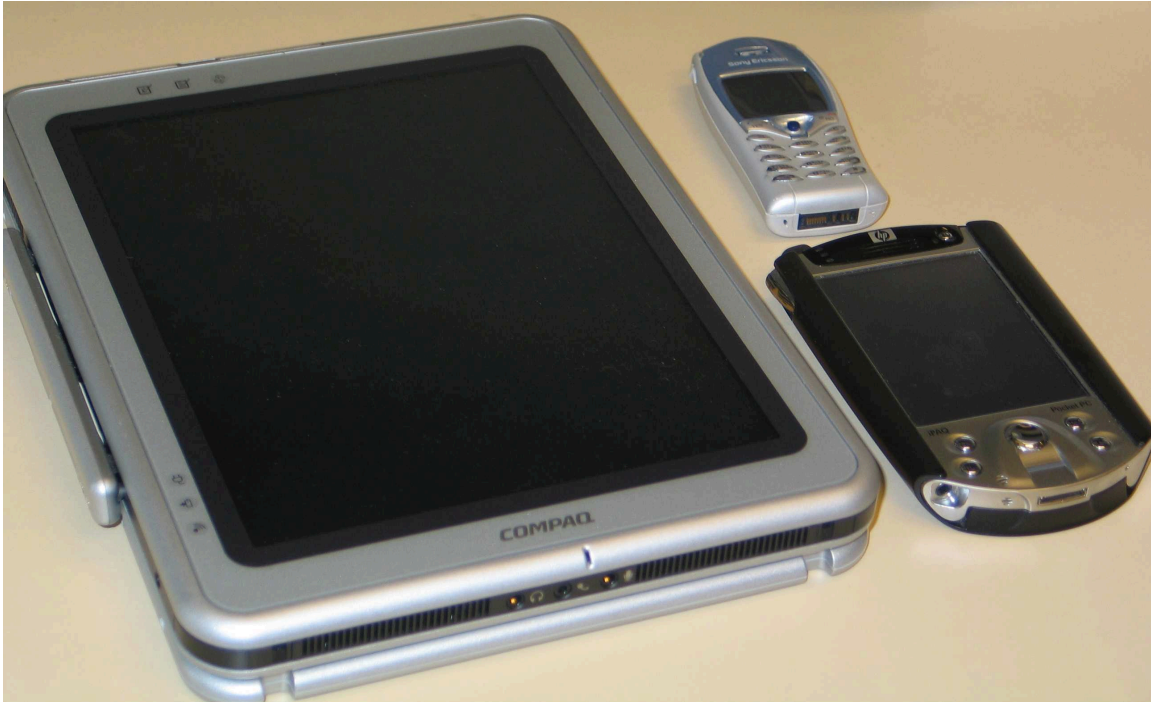
Figure 3.6: A selection of small screens and handheld displays, including PDAs, mobile phones, and Tablet PCs. A chief issue surrounding their effectiveness is the limited amount of display real estate. Unlike desktops or large screens, graphical information like Web pages must be condensed into a representation that loses as little of the original intent as possible.
