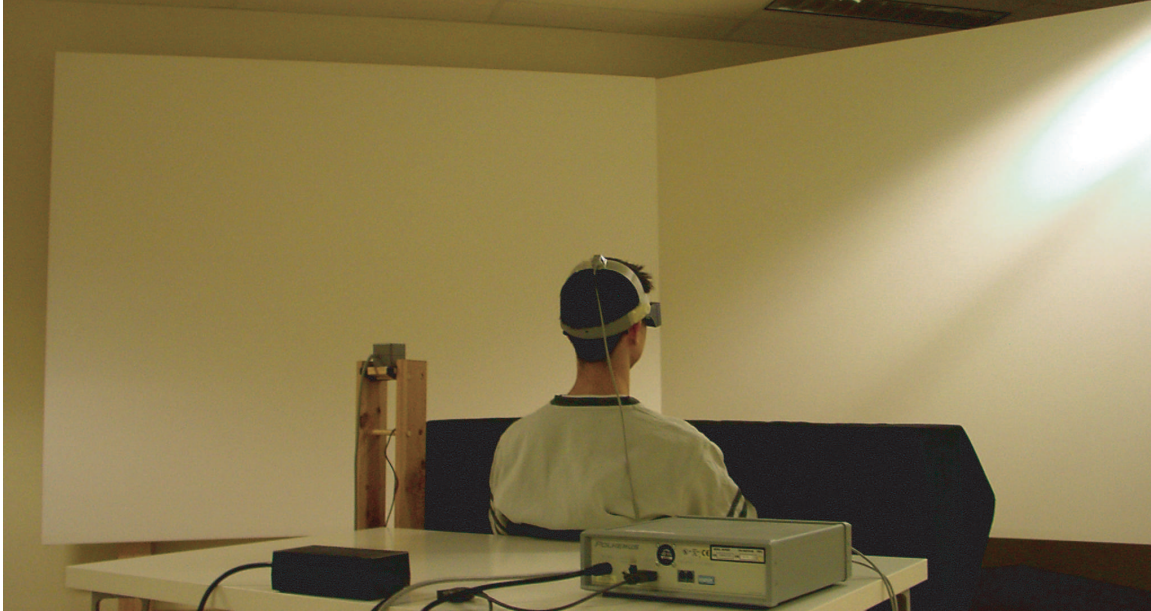
Figure 7.4: A photograph of the large screen display environment used in this experiment. Participants were centered and seated before a three-screen, wide-angle display. Only the center display was used in this study. Pointing interaction was implemented with a Polhemus Fastrak and an attached stylus. Arms and hands were kept beneath a large wooden table at all times. During sessions, all ambient light was extinguished and a researcher was always present.
