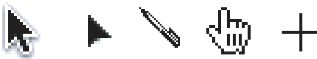
Figure 5.1: Graphical cursors as they appear in several popular GUI-based systems. The most popular pointing cursor in these GUIs is an arrow oriented toward the upper-left corner of the display. Other pointing cursors may not be explicitly shaped as an arrowhead but may convey directional cues nonetheless, such as the “pointing hand” and pen-shaped cursors in the figure. These cursor representations tend to vary little across systems and thus constitute a graphical standard that does not appear to have been extensively evaluated.
