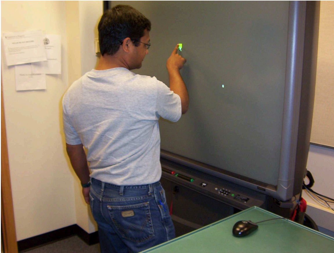
Figure 6.3: A photo of the experimental apparatus used in this experiment. Participants stood upright during each block of trials. In this photo, a participant is selecting items using touch input. In the mouse block of trials, a mouse was placed at a comfortable height on a stable surface to the right-hand side of participants.
