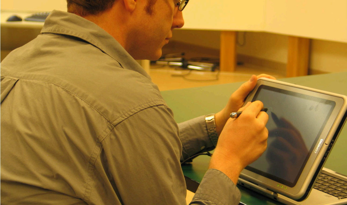
Figure 5.6: The pen condition apparatus used in this experiment. Participants used a Tablet PC and its accompanying pen to select highlighted targets on this portable display. Selection was indicated by directly tapping highlighted items with the pen.
