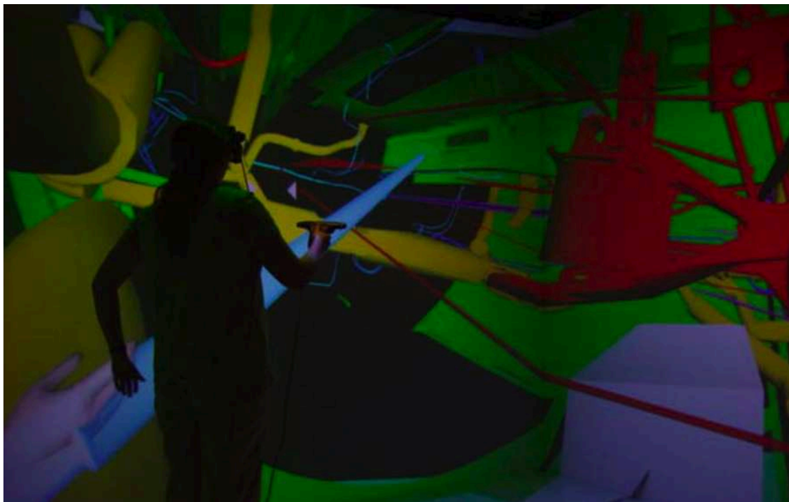
Figure 3.5: A user working inside a CAVE-style multi-screen display environment (Swindells et al., 2004). Large screens are typically used in this fashion as the basis for immersive virtual environments for 3D navigation and wayfinding. These displays are expensive and evidence for their utility remains an open question in HCI. Large screen display configurations differ upon context of use. Some consist only of a single screen while others still are horizontally-oriented in the form of tabletop displays.
