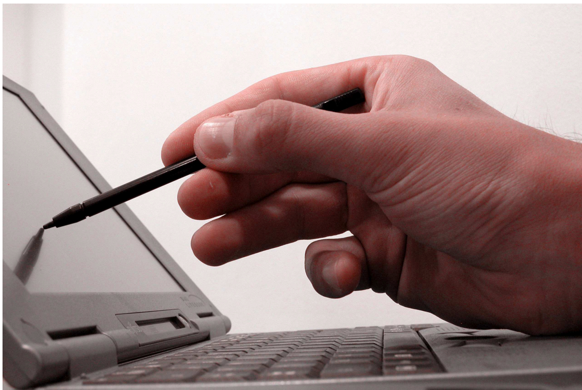
Figure 3.3: An illustration of touchscreen technology at work. Touchscreens and other touch-sensitive displays have become more popular with the increased demand for portable devices, such as mobile phones and PDAs. Touch input primarily differentiates itself from other forms of absolute-mode input by requiring the user to make contact with the display surface (either directly with the finger, or with a physical implement such as a pen or stylus) to indicate interaction.
