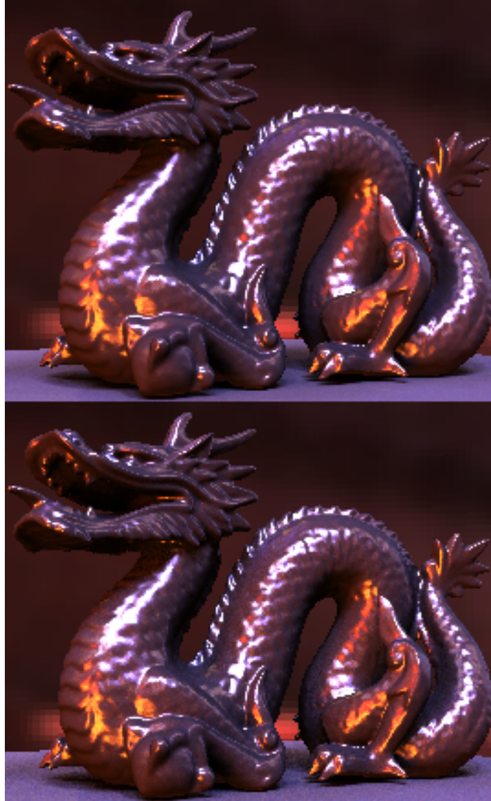
Figure 5.9: Our SIR algorithm compared to the full solution. 268x220 image of the Dragon model (871k triangles) in Grace Cathedral. Top: converged image (hours); Bottom: SIR algorithm using 150/3000 samples (90 sec)
