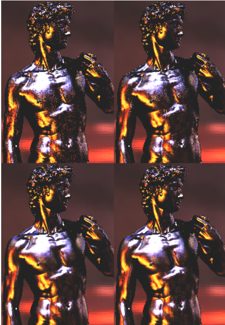
Figure 5.2: David in Grace Cathedral. Phong exp 50, k_s = 1.0 , k_d = 0.0 . 176x248 image rendered in 12.0 seconds. Clockwise from top left: 100 EM samples; 75 BRDF samples; 15/800 rejection samples; 15/800 SIR samples.
