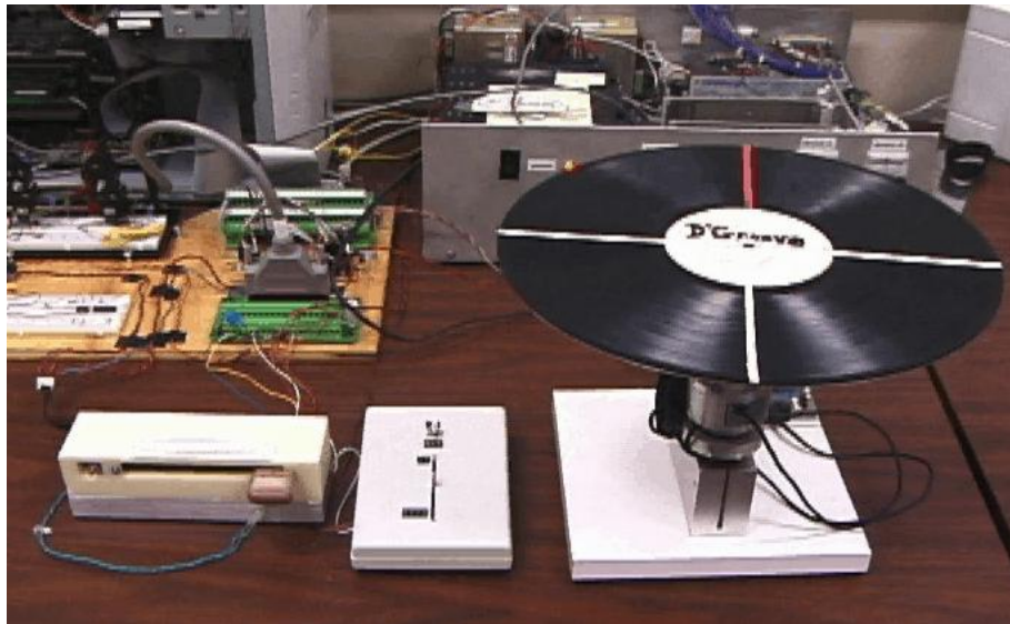
Figure 12 The D'Groove System. From left to right: the Q-slider, the pitch slider, and the turntable.
