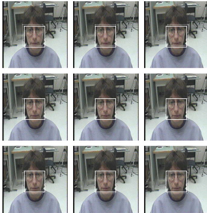
Figure 4-5 Correlation Windows Distribution around Head Position
