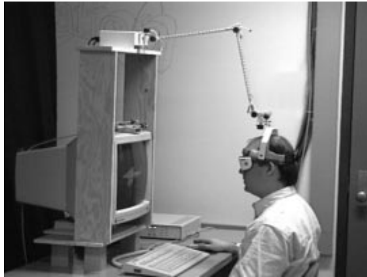
Figure 4.1: The head-coupled stereo display system. The subject's head position is measured by the ADL-1 mechanical tracker. StereoGraphics glasses are worn to provide different images to the left and right eyes, and the display monitor is synchronized with the glasses to provide an effective 60 Hz to each eye.
