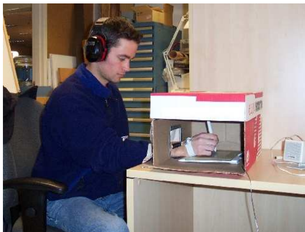
Figure 7: Experimental Setup. Participant is wearing the buzzer on a wristband attached to his wrist. Note the presence of the sound blocking headphones and the occlusion of the participant's view of his hand by the box.
