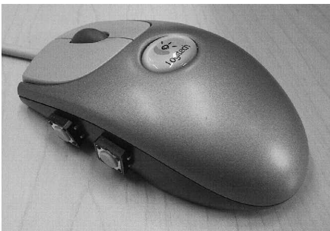
Fig. 4. Modified logitech iFeel mouse with thumb buttons.
