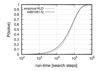
The optimal fit exponential distribution obtained from the Marquardt-Levenberg algorithm passes the  $\chi^2$  goodness-of-fit test at  $\alpha = 0.05$ .
