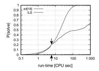
'ed[18]' is the CDF of an exponential distribution with median 18; the arrows mark the optimal cutoff-time for static restarting.
