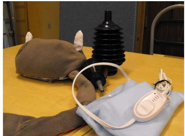
Figure 2: Hapticat device and also the display of the heating pad and the manual breathing mechanism.
