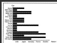
Fig. 11. Incorrect use of a bar chart for the Nation index. The lengths of the bars suggest an ordering on the vertical axis, as if the USA was more popular or better than the other ones, which is not true for the Nation index.
