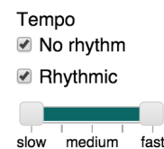
Fig. 4: The tempo filter consists of two checkboxes and a slider to represent the categorical and ordinal nature of tempo attribute.
