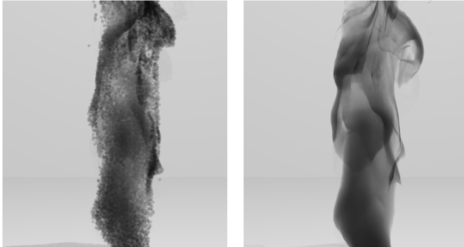
Figure 5.2: A close-up image reveals the difference in quality between surface meshes and marker particles.
