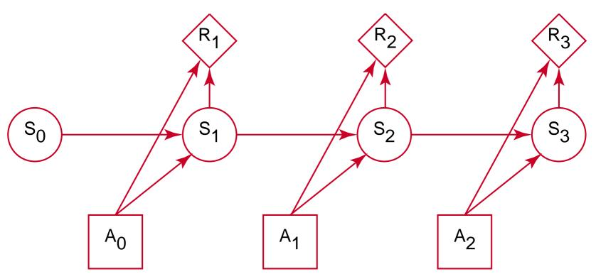
$\frac{P(S_{t+1}|S_t, A_t)}{R(S_t, A_{t-1})}$  specified the dynamics  $\frac{R(S_t, A_{t-1})}{R(S_t, A_{t-1})}$  specifies the reward at time *t* Discounted value is  $R_1 + \gamma R_2 + \gamma^2 R_3 + \dots$
