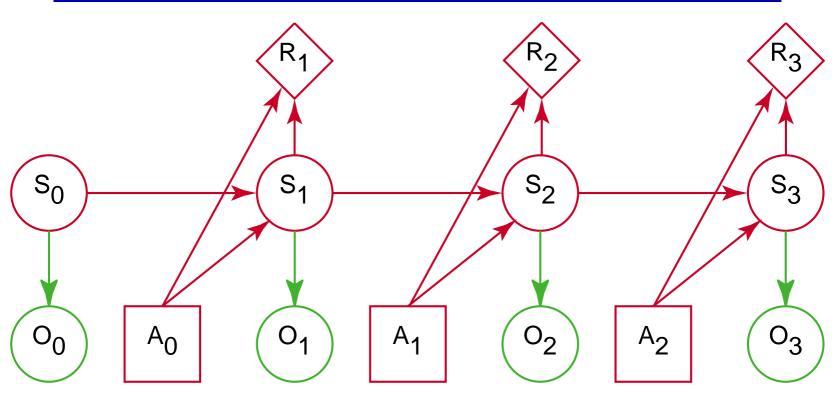
$P(S_{t+1}|S_t, A_t)$ specified the dynamics $P(O_t|S_t)$ specifies the sensor model. $R(S_t, A_{t-1})$ specifies the reward at time *i*
