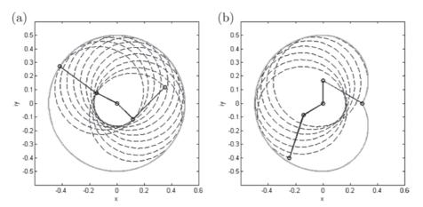
FIG. 2. An illustration of Example 2.3: (a) If a double pendulum with arms of length  $\frac{1}{6}$  and  $\frac{1}{3}$  is allowed to swing freely, it remains inside a disk of radius 0.5. (b) If one arm is constrained to lie in the left half plane, the pendulum swings in the heart-shaped region shown. In both cases the pendulum is unable to reach a set of points surrounding the origin.
