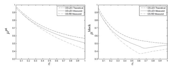
FIG. 5. Theoretical smoothing factors of GS-LEX versus experimental asymptotic convergence rates of two-level multigrid with GS-LEX and GS-RB smoothers, applied to the steady-state diffusion equation  $-u_{xx} - u_{yy} - \varepsilon u_{zz} = f$ . Pointwise relaxation appears on the left, while *x*-oriented line relaxation is depicted on the right. The discretization is on a 23 × 23 × 23 grid with centred differences.
