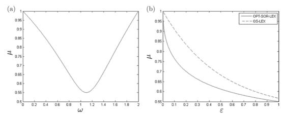
FIG. 4. Left: Smoothing factor of SOR-LEX with relaxation parameter  $\omega$ , as a function of  $\omega$ , for the standard seven-point centred-difference discretization of the three-dimensional Poisson problem. Right: Smoothing factors of GS-LEX and optimal SOR-LEX applied to the anisotropic diffusion problem  $-\varepsilon u_{xx} - u_{yy} - u_{zz} = f$ , as a function of  $\varepsilon$ , assuming seven-point centred-difference discretization.
