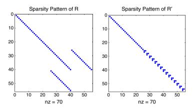
Figure 1. Sparsity patterns of R and R': the original matrix is on the left, and the permuted one is on the right.
