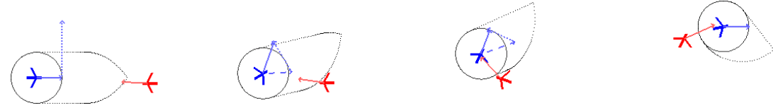
Figure 3.10: Evader keeps pursuer from entering the reachable set, and hence avoids collision (animation at [96]). Note that the shape of the slice of the reachable set depends on the relative heading of the two vehicles.
