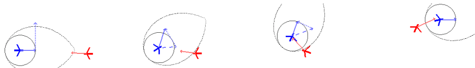
Figure 4.6: Evader keeps pursuer from entering the projective overapproximation \mathcal{Y}_{12} of the reachable set, and hence conservatively avoids collision.
