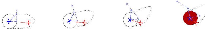
Figure 8: Pursuer starts within the reachable set, and can thus cause a collision despite the best efforts of the evader (animation at [42]).
