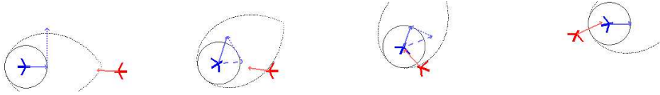
Figure 14: Evader keeps pursuer from entering the projective overapproximation \mathcal{Y}_{12} of the reachable set, and hence conservatively avoids collision.
