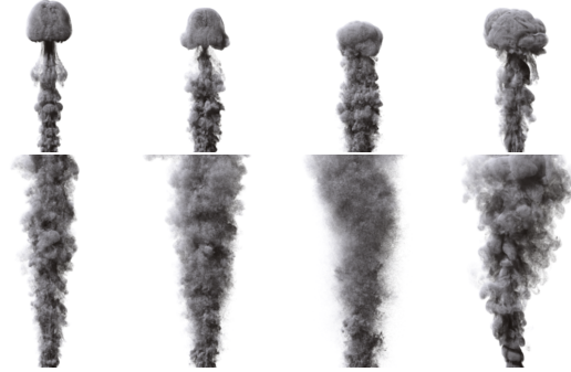
Figure 3: Vorticity confinement (VC) vs. IVOCK. Top row: frame 54 of a rising smoke scenario. From left to right, VC parameter \varepsilon_1 = 0.125 , \varepsilon_2 = 0.25 , \varepsilon_3 = 0.5 , and SL3-IVOCK. Bottom row: frame 162. Vorticity confinement tends to create high-frequency noise everywhere, while IVOCK produces a natural transition from laminar to turbulent flow with realistic vortex structures along the way.
