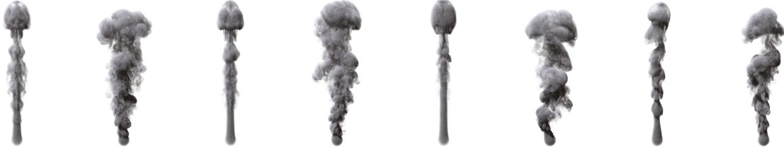
Figure 1: Rising smoke simulations with and without IVOCK (Integrated Vorticity of Convective Kinematics). From left to right: Stable Fluids, Stable Fluids with IVOCK; BFECC, BFECC with IVOCK; MacCormack, MacCormack with IVOCK; FLIP, FLIP with IVOCK.
