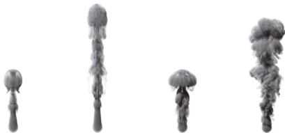
Figure 11: IVOCK can be cheaper and higher quality than taking small time steps. Left and mid-left: BFEC. Mid-right and right: BFEC-IVOCK with twice as large a time step, computed in much less time.
