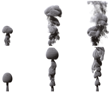
Figure 6: Two sequences from 3D rising smoke simulations. Top row: MC-IVOCK with vortex stretching. Bottom row: MC-IVOCK with vortex stretching switched off. With vortex stretching, vortex rings change their radius under the influence of other vortex rings, these process can easily perturb the shape of vortex rings, breaking them to form new vortex structures, which brings rich turbulence into the flow field.
