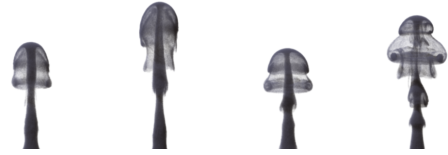
Figure 8: Vortex stretching enhances vortical motion, captured more accurately with IVOCK. Transparent renderings illustrate the internal structures. Left and middle-left: FLIP. Middle-right and right most: FLIP-IVOCK.
