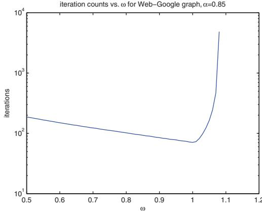
FIG. 6.3. *SOR convergence for the Web-Google matrix: The number of iterations it took to reach a tolerance of  $10^{-10}$  in terms of the  $\ell_1$ -norm of iterate difference for  $\omega = [0.50 : 0.01 : 1.08]$ .*
