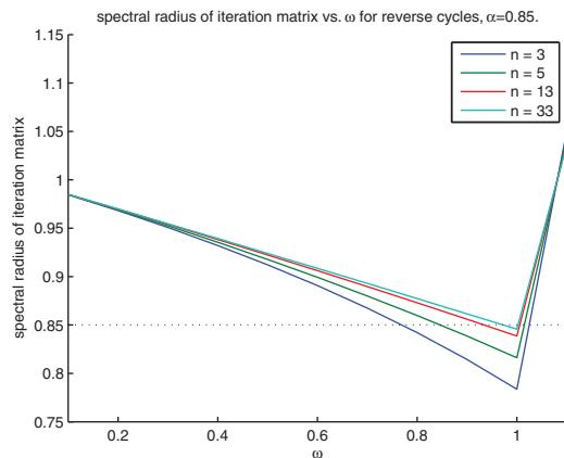
FIG. 6.2. Spectral radius of the SOR iteration matrix versus the relaxation parameter  $\omega$  for reverse odd cycles of various sizes.
