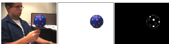
Figure 3: Locating the projection of surface dots. From left: Input; Restricted Input; Ellipses found for red (filled) and green (unfilled) dots.
