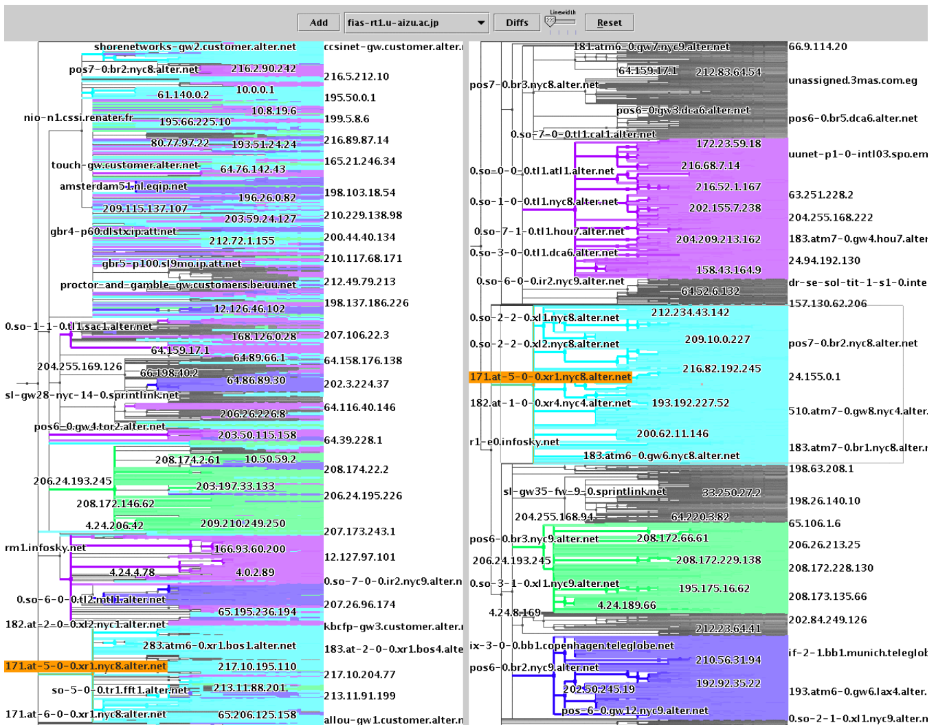
Figure 8: Internet backbone router spanning tree, with topologies inferred from two sources: UDP/traceroute on the left (137,000 nodes) and ICMP/ping (140,000 nodes) on the right. Marking subtrees shows that the two different packet types can take very different routes.
