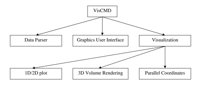
Figure 1 . The architecture of VisCMD
