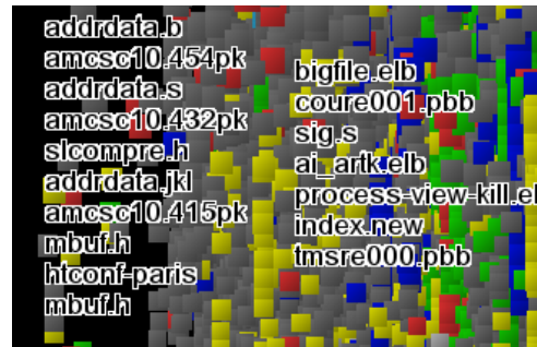
Figure 7: Dynamic Labeling of a Treemap (detail). When clicking on the treemap, labels are displayed dynamically on the outside of the region, which is grayed out. The popup menu allows users to adjust the depth of the region of interest.
