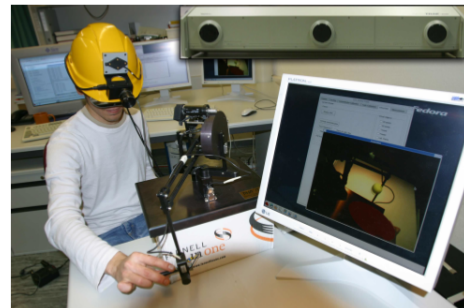
Figure 28: AR haptic feedback apparatus used by Bianchi et al. The optical tracker is shown in the inset [4].
