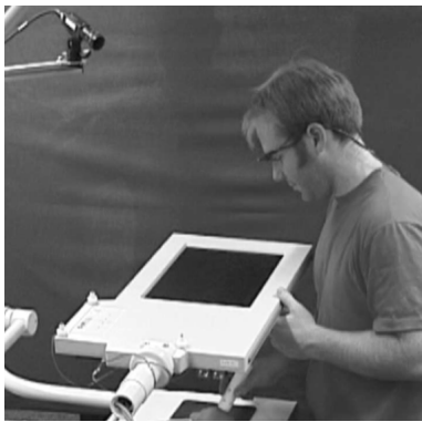
Figure 12: The AR Window is a semi-transparent display that uses eye-tracking technology to superimpose virtual image data on the surgeon's field of view [25].
