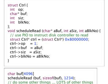
Read is finished when disk controller interrupts CPU
