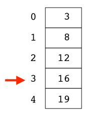
It takes 4 passes through the array to get it completely sorted. There are 4 comparisons on the first pass, 3 comparisons on the second pass, 2 comparisons on the third pass, and 1 comparison on the last pass. That is, it takes 4 + 3 + 2 + 1 = 10 comparisons to sort an array of five values.
