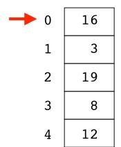
We can go back to the selection sort example and count the comparisons. The first pass through the array of 5 elements started with 16 being compared to 3, then 3 was compared to 19, 8, and 12. There were 4 comparisons. The value 3 was moved into the location at index 0.
