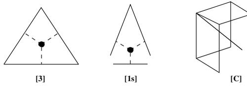
Figure 4: Special Voronoi edges and their projections. [3] Edge with governor entities which are adjacent in pairs. [1s] Edge with two adjacent governors, with a sharp angle between them. [C] A Voronoi diagram edge, which is not interior (the edge is shown as the thin line starting in the corner).
