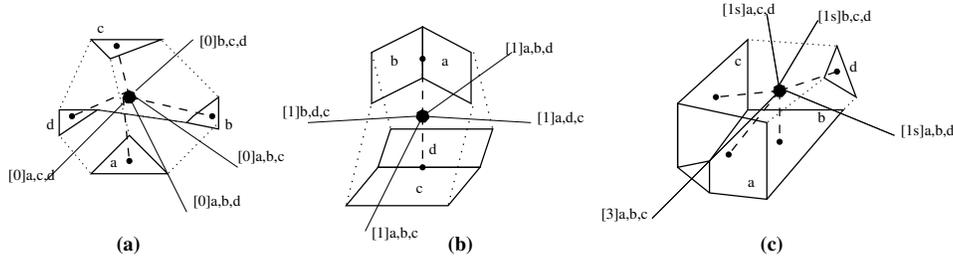
Figure 6: Projection of vertices. The entities of the volume are shown in bold. The edges are shown as thin lines, and the vertex projections are shown as dashed lines. In (a) the projections implied by the edges are identical. In (b) the projections implied by the edges are adjusted to match. In (c) the edge projections are changed so they can match (from [1] to [1s]).
