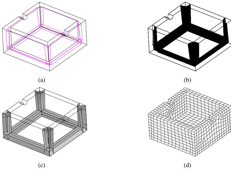
Figure 18: Mesh of an ashtray shape: (a) The initial volume with the embedded Voronoi graph. (b) The decomposition faces generated based on the embedded Voronoi graph, using only Voronoi edges with two or more face governors. (c) The decomposition faces generated based on the embedded Voronoi graph, using all interior Voronoi edges. (d) Mesh of the volume (after merging groups of sub-volumes). The mesh contains 1226 elements.
