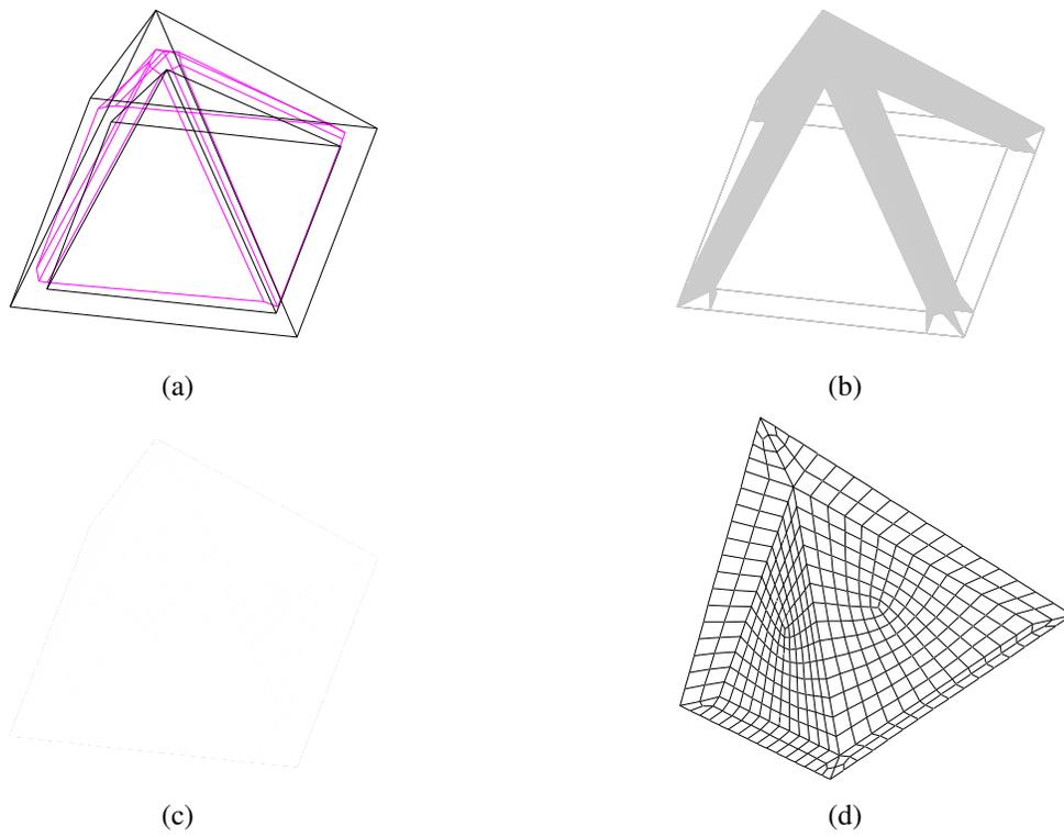
Figure 16: Mesh of a hollow pyramid: (a) The initial volume with the embedded Voronoi graph. (b) The decomposition faces generated based on the embedded Voronoi graph. (c) Mesh of the pyramid (before smoothing). The mesh contains 1472 elements. (d) Mesh of half the pyramid, view from inside.
