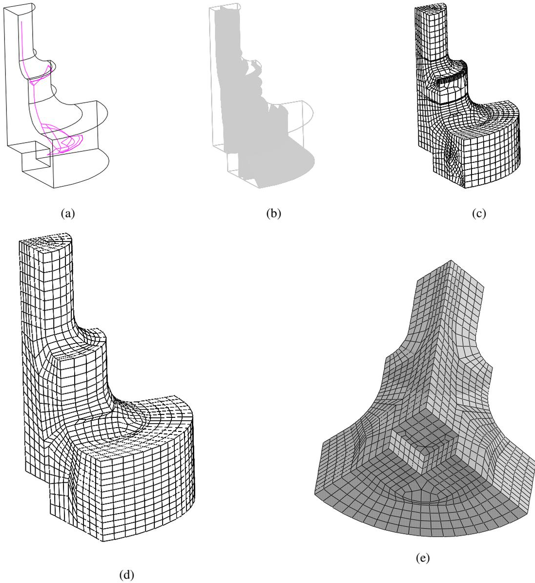
Figure 14: A meshing example: (a) The initial volume with the embedded Voronoi graph. (b) The decomposition faces generated based on the embedded Voronoi graph. (c) Mesh of the set of volumes, generated by the decomposition. (d) Mesh of a set of volumes, after merge of several volumes, to improve mesh quality (front view). The mesh contains 3625 elements. (e) Mesh of a set of volumes after merge (back view).
