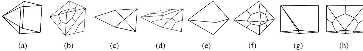
Figure 10: Template meshes of some common sub-volumes. Note that using the template mesh, prevents sweeping along the quad faces in the adjacent volumes. (a,b) A sub-volume generated by projecting a Voronoi edge to two governor faces sharing a vertex. (c,d) A volume shaped as a union of two tetrahedra (generated by projecting a Voronoi edge to two adjacent governor edges). (e,f) (g,h) Two types of sub volumes generated at [C] vertices, with edge governors.
