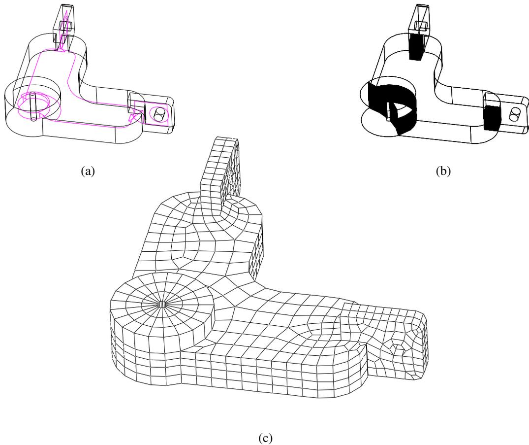
Figure 17: Mesh of a support arm: (a) The initial volume with the embedded Voronoi graph. (b) The decomposition faces generated based on the embedded Voronoi graph(only Voronoi edges with two or more face governors were used). (c) Mesh of the arm. It contains 1259 elements.
