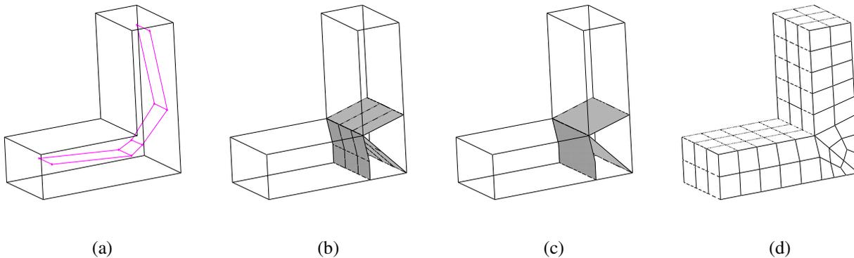
Figure 1: The stages of the meshing algorithm applied on an ‘L’ shaped volume: (a) the embedded Voronoi graph (only interior entities are shown); (b) the decomposition faces, generated by the projection of Voronoi edges and vertices; (c) The decomposition of the volume into four sub-volumes, showing the decomposition faces after they were merged; (d) the resulting volume mesh (before smoothing).
