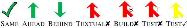
Figure 8: Crystal associates an icon with each of the seven relationships. The color of each relationship icon represents the severity of the relationship (Section 3.2): relationships that require no merging are green, that can be merged automatically are yellow, and that require manual merging are red.
