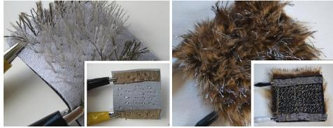
Figure 2: Buechley’s conductive thread stroke sensor (left) [5], our conductive fur touch and gesture sensor (right).
