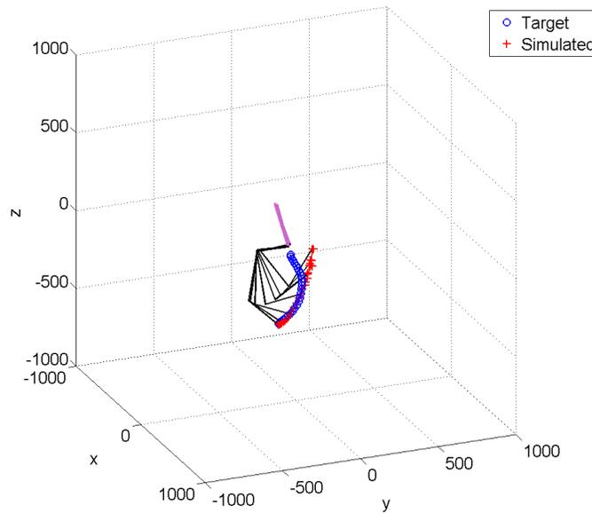
Figure 3: Inverse kinematic result on a trajectory in the test set.
