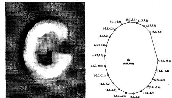
Figure 3: On the left is an image of the G-shaped part, on the right its 20 vertex model.
