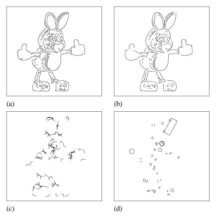
Figure 4: Features of a bunny training image. Shown here are selected features found in the  $0^{\circ}$  elevation,  $10^{\circ}$  azimuth training image (right image in figure 3). (a) Edgels. (b) Curve features. (c) L-junction features. (d) Parallel-curve features (depicted by parallel lines), Region features (depicted by rectangles), and Ellipse features (depicted by circles).
