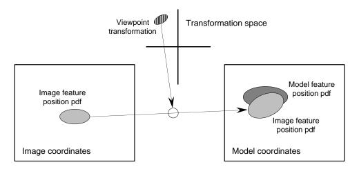
Figure 2: Comparison of image and model feature positions. An image feature's position is transformed from image coordinates (*left*) to model coordinates (*right*) according to an estimate of the viewpoint transformation. Uncertainty in the positions and the transformation are characterized by Gaussian distributions that are compared in the model coordinate space.
