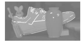
Figure 12: Shoe recognition example. *Left:* Test image. *Right:* Image curve features included in a match to shoe model.
