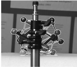
Figure 9: Example showing recognition of a complex object with substantial occlusion. *Left:* One of several training images. *Right:* Image curve features included in the match.
