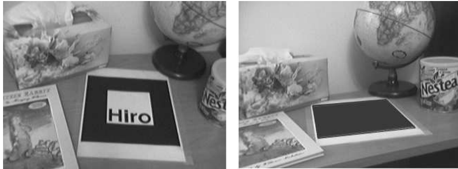
Figure 5.11: ARToolkit marker in the scene (left). Virtual square, superimposed onto the marker during tracking (right).
