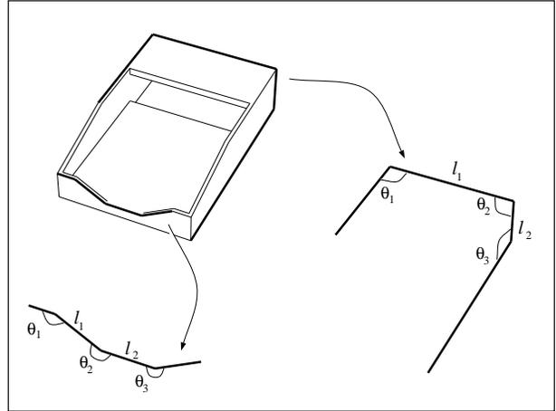
Figure 1:  $N$ -segment chains as examples of Local Feature Sets (with  $N = 4$ ). This type of grouping generates feature vectors  $\vec{x} = (\theta_1, \theta_2, \theta_3, l_2/l_1)$ .
