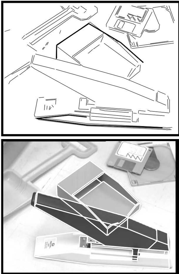
Figure 2: The upper box shows the processed image with the groupings that correctly indexed the model database. The lower box contains the final determination of object poses, overlaid on the original image.
