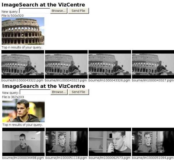
Figure 11. Top: An example of searching the one million image database including all the frames of seven movies and 6376 ground truth images. Searching for a region-rich rigid object such as a CD-cover, book, building or location works quite well even for this size of database. The colosseum search easily finds the frames from a short clip in The Bourne Identity . However, searching for example on faces is less reliable. A lucky shot is shown on the bottom. This search was performed on a smaller database size of 300K frames. Both searches were performed with images separate from the movies.
