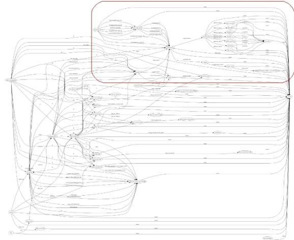
Figure 2. A visualization of the software architecture for Curious George. Each oval represents a single distributed process and arcs between ovals represent data topics that allow the processes to communicate.
