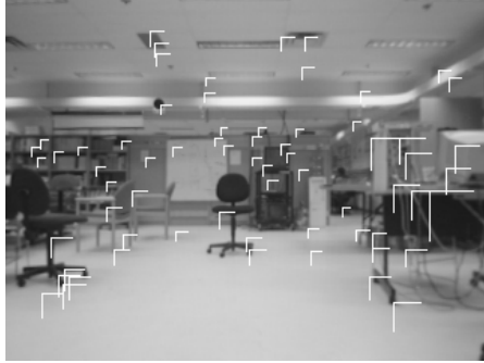
Figure 1: SIFT stereo matching result, where horizontal and vertical lines indicate the horizontal and vertical disparities respectively.
