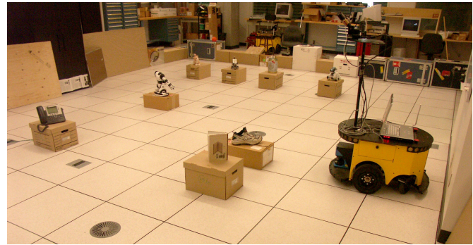
Fig. 1. The handcrafted experimental setup for accurately assessing the informed visual search technique. The robot has models of a number of objects, and searches for them in a previously unknown environment during a limited time.
