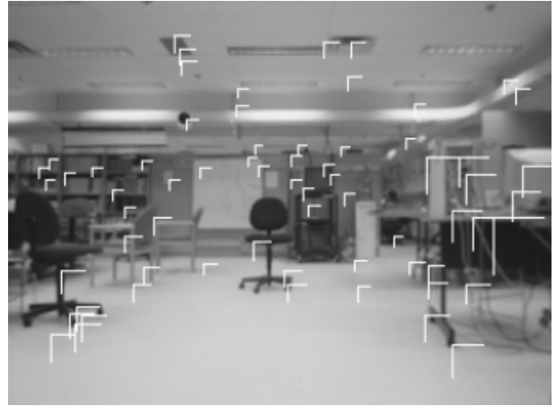
Fig. 1. SIFT features found by our stereo-equipped robot. SIFT features in the three stereo images are matched; horizontal and vertical lines indicate the horizontal and vertical disparities respectively (from [17]).
