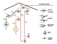
Similarly, W0 depends only on whether there is power in w1, whether there is power in w2, the position of switch s2 ( $S2_pos$ ), and the status of switch s2 ( $S2_st$ ).
