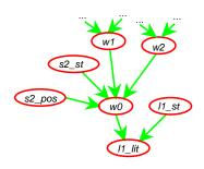
Similarly, W0 depends only on whether there is power in w1, whether there is power in w2, the position of switch s2 ( $S2\_pos$ ), and the status of switch s2 ( $S2\_st$ ).
