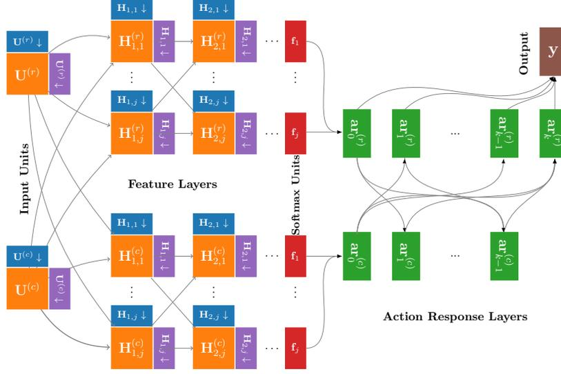
Figure 2: A schematic representation of our architecture. The feature layers consist of *hidden matrix units* (orange), each of which use *pooling units* to output row- and column-preserving aggregates (blue and purple) before being reduced to distributions over actions in the *softmax units* (red). Iterative response is modeled using the *action response layers* (green) and the final output,  $y$ , is a weighted sum of the row player’s action response layers.
